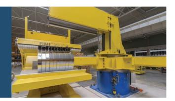
Exit coil car with different configurations for off-line strapping.
