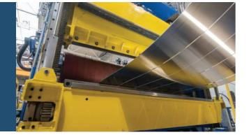
Automatic solutions for cutting of coil tails and for the division of the coils into baby coils with rapid resumption of processing.
