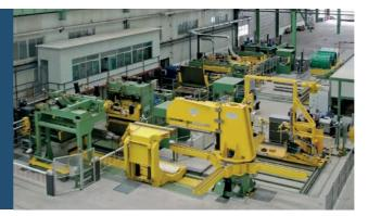
Slitting Lines for Hot Rolled Heavy Gauge Steel have been successfully developed to match the typical applications in structural engineering, cranes, lifting equipment in general, poles for wind turbines and for the pipes & tubes industry. The thickness range is from 2 to 20 m. These Slitting Lines require special solutions for the strip feeding process especially after the slitting shear, for scrap chopping and handling, for strip recoiling and discharge.
