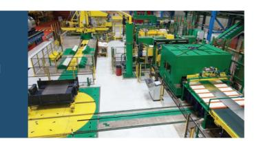
Recoiling & Coil Inspection Lines are required mainly in the Automotive Industry to check the quality of the material surfaces, but they find application also in the Rolling Mills to reduce the size of rolled coils, divide the coils in length, check the surfaces.
