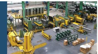
Special Slitting Line configuration for processing high and ultra-high strength material, up to 2.000 Mpa tensile value.
