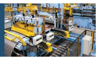
Slitting Lines for automotive applications are especially designed to fulfil the surface quality needs, cutting precision and quality required by car manufacturers. The typical thickness range is 0,3-3 mm, but it goes up to 8 mm in the case of car structural steels.
