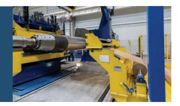
Slits Threading Grippers from Slitting Shear to Recoiler Mandrel
