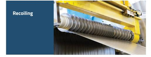
Winding from above and below, with or without clamping. Solutions dedicated to avoid marking sensitive materials.
